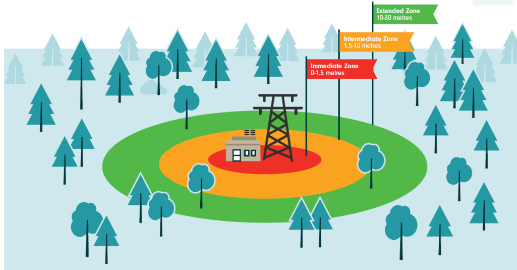
Figure 7: FireSmart Home and Critical Infrastructure Ignition Zone (HIZ, CIIZ)
