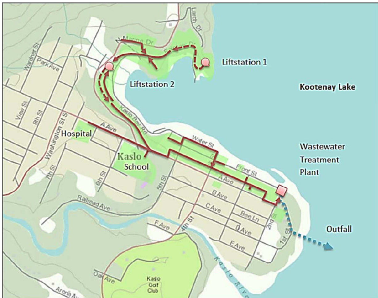
Figure 1. Village of Kaslo and location of wastewater treatment plant and outfall
